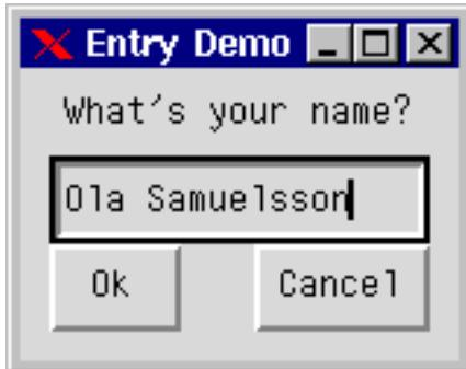
Figure 8.4: Label and Entry Objects for User Input
