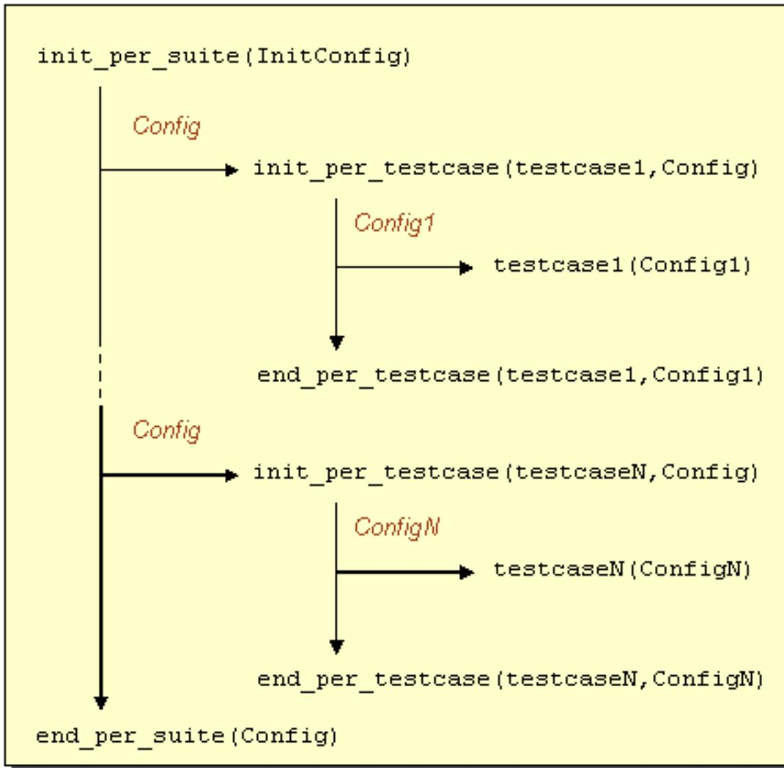
**Figure .2:** Config data flow in the suite.
