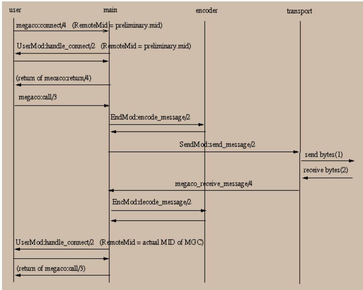
Figure 3.3: MG Startup Call Flow (no MID)
